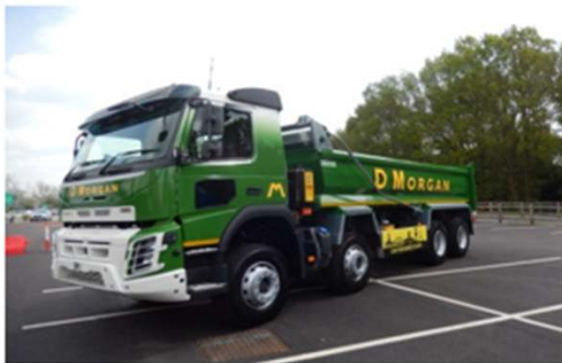
8 wheeler 32 tonne GVW Construction tipper
